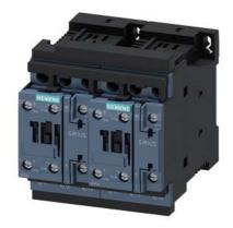
reversing contactor assembly, AC-3e/AC-3, 32 A, 15 kW / 400 V, 3-pole, 24 V DC, screw terminal, electrical and mechanical interlock, auxiliary contacts: 2 x 1 NO
