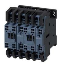
reversing contactor assembly, AC-3e/AC-3, 12 A, 5.5 kW / 400 V, 3-pole, 24 V AC, 50/60 Hz, spring-loaded terminal, electrical and mechanical interlock, auxiliary contacts: 2 x 1 NO
