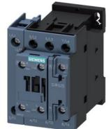
contactor AC-1, 50 A, 400 V / 40 °C, 4-pole, 24 V AC, 50 Hz, auxiliary contacts: 1 NO + 1 NC, screw terminal, size: S0
