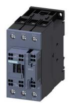
power contactor, AC-3e/AC-3, 51 A, 22 kW / 400 V, 3-pole, 230 V AC, 50 Hz, auxiliary contacts: 1 NO + 1 NC, main circuit: screw terminal, control and auxiliary circuit: spring-loaded terminal, size: S2, upright mounting position
