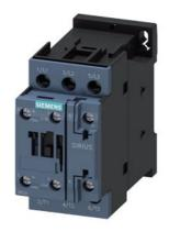
power contactor, AC-3e/AC-3, 32 A, 15 kW / 400 V, 3-pole, 230 V AC, 50/60 Hz, auxiliary contacts: 1 NO + 1 NC, screw terminal, size: S0, upright mounting position
