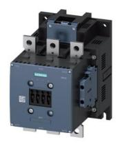
power contactor, AC-3e/AC-3 225 A, 110 kW / 400 V AC (50-60 Hz) / DC Uc: 96-127 V PLC input 24 V DC 3-pole, auxiliary contacts 2 NO + 2 NC drive: electronic main circuit: busbar control and auxiliary circuit: screw terminal
