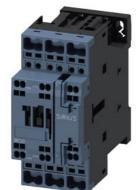
power contactor, AC-3e/AC-3, 32 A, 15 kW / 400 V, 3-pole, 24 V AC, 50 Hz, auxiliary contacts: 1 NO + 1 NC, spring-loaded terminal, size: S0
