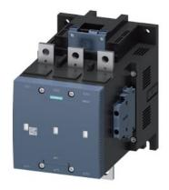
vacuum contactor AC-3e/AC-3 500 A, 250 kW / 400 V, 3-pole, Uc: 21-27.3 V AC(50-60 Hz) / DC PLC input 24 V DC drive: electronic auxiliary contacts 2 NO + 2 NC main circuit: busbar control and auxiliary circuit: screw terminal
