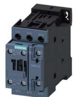
power contactor, AC-3e/AC-3, 38 A, 18.5 kW / 400 V, 3-pole, 48 V DC, auxiliary contacts: 1 NO + 1 NC, screw terminal, size: S0
