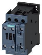
power contactor, AC-3e/AC-3, 38 A, 18.5 kW / 400 V, 3-pole, 24 V AC, 50/60 Hz, auxiliary contacts: 1 NO + 1 NC, screw terminal, size: S0, India 40 A, Tu max. 50  $^\circ\text{C}$
