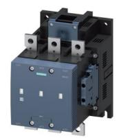
vacuum contactor AC-3e/AC-3 300 A, 160 kW / 400 V, 3-pole, Uc: 240-277 V AC(50-60 Hz) / DC drive: conventional auxiliary contacts 2 NO + 2 NC main circuit: busbar control and auxiliary circuit: screw terminal
