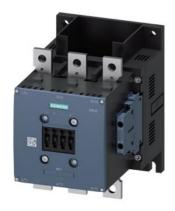
power contactor, AC-3e/AC-3 300 A, 160 kW / 400 V, without operating mechanism 3-pole, auxiliary contacts 2 NO + 2 NC main circuit: busbar control and auxiliary circuit: screw terminal
