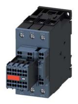
power contactor, AC-3e/AC-3, 41 A, 18.5 kW / 400 V, 3-pole, 230 V AC, 50/60 Hz, with plugged-in varistor, auxiliary contacts: 2 NO + 2 NC, main circuit: screw terminal, control and auxiliary circuit: spring-loaded terminal, size: S2, captive auxiliary switch
