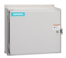
Mechanically held lighting contactor, Contactor amp rating 30A, 0 N.C. / 6 N.O. poles, 277VAC 60HZ coil, Non-combination type, Enclosure NEMA type 12, Dust/drip proof for indoors
