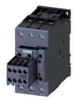
power contactor, AC-3e/AC-3, 51 A, 22 kW / 400 V, 3-pole, 230 V AC, 50 Hz, auxiliary contacts: 2 NO + 2 NC, screw terminal, size: S2, removable auxiliary switch
