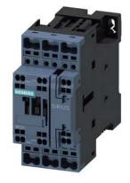
traction contactor, AC-3e/AC-3, 38 A, 18.5 kW / 400 V, 3-pole, 72 V DC, 0.7-1.25\* Us, electronic drive, with integrated varistor, auxiliary contacts: 1 NO + 1 NC, spring-loaded terminal, size: S0
