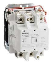
Mechanically held lighting contactor, Contactor amp rating 200A, 0 N.C. / 5 N.O. poles, 208VAC 60HZ coil, Non-combination type, Enclosure NEMA type (open), No enclosure
