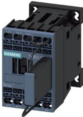
traction contactor, AC-3e/AC-3, 12 A, 5.5 kW / 400 V, 3-pole, 110 V DC, 0.7-1.25\* Us, with integrated varistor, auxiliary contacts: 1 NC, spring-loaded terminal, size: S00, with plugged on series resistor, upright mounting position
