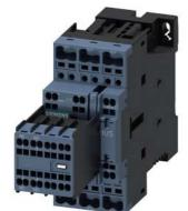
power contactor, AC-3e/AC-3, 25 A, 11 kW / 400 V, 3-pole, 110 V DC, auxiliary contacts: 2 NO + 2 NC, spring-loaded terminal, size: S0, removable auxiliary switch
