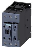
power contactor, AC-3e/AC-3, 51 A, 22 kW / 400 V, 3-pole, 230 V AC, 50/60 Hz, auxiliary contacts: 1 NO + 1 NC, screw terminal, size: S2, upright mounting position
