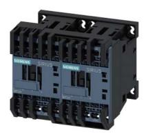
reversing contactor assembly, AC-3e/AC-3, 9 A, 4 kW / 400 V, 3-pole, 24 V AC, 50/60 Hz, spring-loaded terminal, electrical and mechanical interlock
