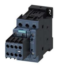
power contactor, AC-3e/AC-3, 17 A, 7.5 kW / 400 V, 3-pole, 24 V DC, with plugged-in diode combination, auxiliary contacts: 3 NO + 2 NC, screw terminal, size: S0, with 3RH2911-1HA21
