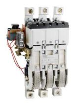
Mechanically held lighting contactor, Contactor amp rating 300A, 0 N.C. / 2 N.O. poles, 110VAC 50HZ/120VAC 60HZ coil, Non-combination type, Enclosure NEMA type (open), No enclosure
