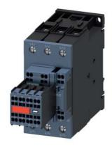
power contactor, AC-3e/AC-3, 41 A, 18.5 kW / 400 V, 3-pole, 110 V AC, 50 Hz / 120 V, 60 Hz, auxiliary contacts: 2 NO + 2 NC, main circuit: screw terminal, control and auxiliary circuit: spring-loaded terminal, size: S2, captive auxiliary switch
