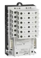
Electrically held lighting contactor, (convertible to mech. held), Amp rating 30A (tungsten 20A), 2 N.C. / 2 N.O. poles, 347V 60Hz coil, Non-combination type, Enclosure NEMA type (open), No enclosure
