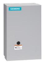
Mechanically held lighting contactor, Contactor amp rating 100A, 0 N.C. / 5 N.O. poles, 24VAC 60HZ coil, Non-combination type, Enclosure NEMA type 1, Indoor general purpose use
