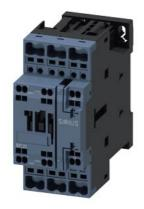
power contactor, AC-3e/AC-3, 25 A, 11 kW / 400 V, 3-pole, 480 V AC, 60 Hz, with plugged-in varistor, auxiliary contacts: 1 NO + 1 NC, spring-loaded terminal, size: S0
