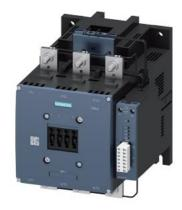
power contactor AC-1 690 A / 690 V / 40  $^{\circ}$ C 3-pole, Uc: 200-277 V AC(50-60 Hz) / DC PLC input 24 V DC drive: electronic auxiliary contacts 2 NO + 2 NC main circuit: busbar control and auxiliary circuit: screw terminal with remaining lifetime indicator
