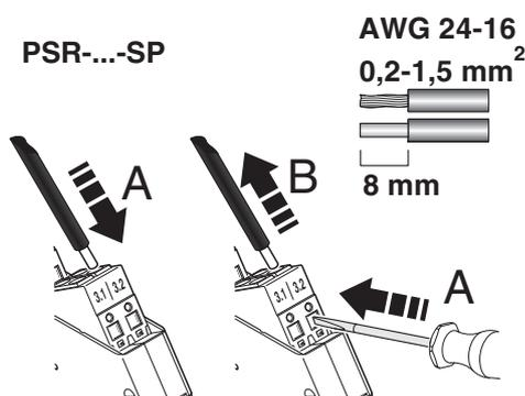
Figure 8 Connecting the cables for PSR-...-SC (spring-cage terminal block)
