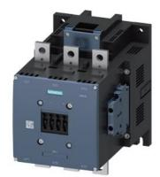
power contactor AC-1 690 A / 690 V / 40  $^\circ$ C 3-pole, Uc: 42-48 V AC(50-60 Hz) / DC drive: conventional auxiliary contacts 2 NO + 2 NC main circuit: busbar control and auxiliary circuit: screw terminal
