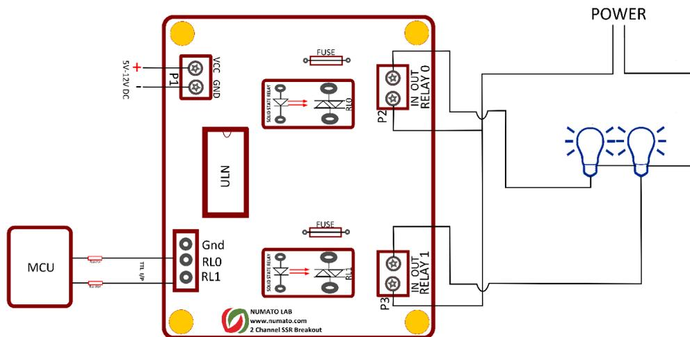
Above image shows basic connection diagram that can be used in most of the situations. The connection diagram showed above is for AC load. Please make sure to use a freewheeling diode or snubber circuit if the load is inductive.
