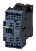
power contactor, AC-3e/AC-3, 17 A, 7.5 kW / 400 V, 3-pole, 125 V DC, 0.7-1.25  $^{\star}$  Us, with plugged-in varistor, auxiliary contacts: 1 NO + 1 NC, spring-loaded terminal, size: S0, suitable for PLC outputs, not expandable with auxiliary switch
