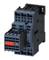
power contactor, AC-3e/AC-3, 38 A, 18.5 kW / 400 V, 3-pole, 230 V AC, 50/60 Hz, with plugged-in varistor, auxiliary contacts: 2 NO + 2 NC, spring-loaded terminal, size: S0, captive auxiliary switch
