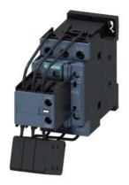
capacitor contactor, AC-6b 20 kVAr, / 400 V, 3-pole, 24 V AC, 50 Hz, auxiliary contacts: 1 NO + 2 NC, screw terminal, size: S0  $\,$
