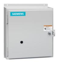
Mechanically held lighting contactor, Contactor amp rating 60A, 0 N.C. / 2 N.O. poles, 110VAC 50HZ/120VAC 60HZ coil, Non-combination type, Enclosure NEMA type 12, Dust/drip proof for indoors
