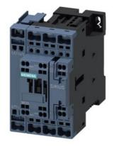
contactor AC-1, 40 A, 400 V / 40  $^{\circ}$ C, 4-pole, 24 V DC, auxiliary contacts: 1 NO + 1 NC, spring-loaded terminal, size: S0
