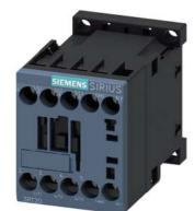
power contactor, AC-3e/AC-3, 12 A, 5.5 kW / 400 V, 3-pole, 24 V DC, auxiliary contacts: 1 NO, screw terminal, size: S00
