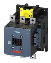
power contactor, AC-3e/AC-3 300 A, 160 kW / 400 V, AC (50-60 Hz) / DC 200-277 V x (0.8-1.1) F-PLC input 24 V DC 3-pole, auxiliary contacts 2 NO + 2 NC permanently mounted drive: electronic main circuit: busbar control and auxiliary circuit: screw terminal
