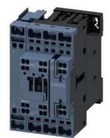
power contactor, AC-3, 25 A, 11 kW / 400 V, 4-pole, 230 V AC, 50 Hz, main contacts: 2 NO + 2 NC, auxiliary contacts: 1 NO + 1 NC, spring-loaded terminal, size: S0
