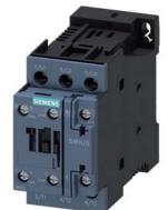
power contactor, AC-3e/AC-3, 32 A, 15 kW / 400 V, 3-pole, 60 V DC, auxiliary contacts: 1 NO + 1 NC, screw terminal, size: S0
