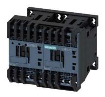
reversing contactor assembly, AC-3e/AC-3, 16 A, 7.5 kW / 400 V, 3-pole, 24 V DC, spring-loaded terminal, electrical and mechanical interlock, with voltage tap for  $3 \rm RA27$
