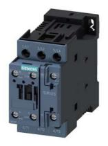
power contactor, AC-3e/AC-3, 9 A, 4 kW / 400 V, 3-pole, 24 V DC, auxiliary contacts: 1 NO + 1 NC, screw terminal, size: S0, communication-capable
