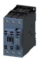
power contactor, AC-3e/AC-3, 65 A, 30 kW / 400 V, 3-pole, 20-33 V AC/DC, 50/60 Hz, with integrated varistor, auxiliary contacts: 1 NO + 1 NC, main circuit: screw terminal, control and auxiliary circuit: spring-loaded terminal, size: S2, communication-capable
