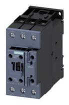
contactor, NEMA version, 25 HP, 460 / 575 V, 3-pole, 220 V AC, 50 Hz / 240 V, 60 Hz, auxiliary contacts: 1 NO + 1 NC, screw terminal, size: S2  $\,$
