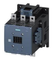
power contactor, AC-3e/AC-3 400 A, 200 kW / 400 V AC (50-60 Hz) / DC Uc: 240-277 V 3-pole, auxiliary contacts 2 NO + 2 NC drive: conventional main circuit: busbar control and auxiliary circuit: screw terminal
