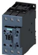
power contactor, AC-3e/AC-3, 51 A, 22 kW / 400 V, 3-pole, 20-33 V AC/DC, 50/60 Hz, with integrated varistor, auxiliary contacts: 1 NO + 1 NC, screw terminal, size: S2, communication-capable
