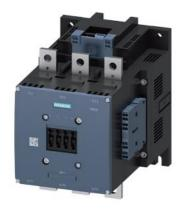
power contactor, AC-3e/AC-3 400 A, 200 kW / 400 V Uc: 72 V DC x (0.7-1.25) PLC input 24-110 V DC 3-pole, auxiliary contacts 2 NO + 2 NC drive: electronic main circuit: busbar control and auxiliary circuit: spring-loaded terminal extended rated condition railroad IEC 60077
