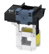
Withdrawable drive for contactors 3RT105, 3RT145 AC (50...60 Hz) / DC operation, 200 ... 277 V Operating mechanism: electronic with PLC input 24 V DC Spring-type terminal
