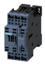
power contactor, AC-3, 25 A, 11 kW / 400 V, 4-pole, 125 V DC, main contacts: 2 NO + 2 NC, auxiliary contacts: 1 NO + 1 NC, spring-loaded terminal, size: S0
