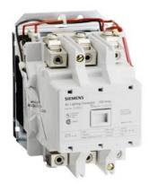
Mechanically held lighting contactor, Contactor amp rating 100A, 0 N.C. / 5 N.O. poles, 208VAC 60HZ coil, Non-combination type, Enclosure NEMA type (open), No enclosure
